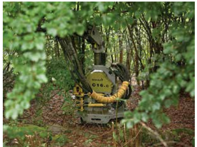
Bracke C16.c, accumulating felling head for silviculture and biomass applications.
