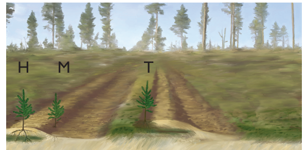
The Bracke T28.a creates planting spots with inverted humus (T), mineral soil mounds on inverted humus (H), and mineral soil mounds (M).
