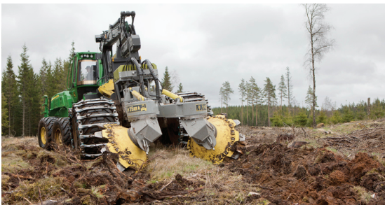
The Bracke T28.a is mounted on a medium-sized or large prime mover.
