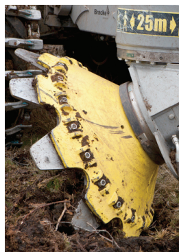
Discs with replaceable teeth.
