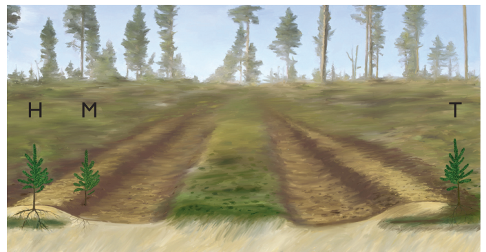
The Bracke T26.b creates planting spots with inverted humus (T), mineral soil mounds on inverted humus (H), and mineral soil mounds (M).
