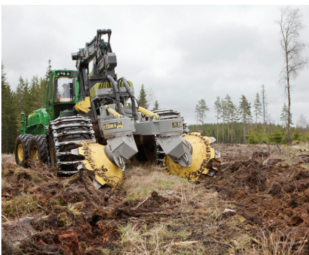
The Bracke T26.b attaches to medium-sized or large prime movers.
