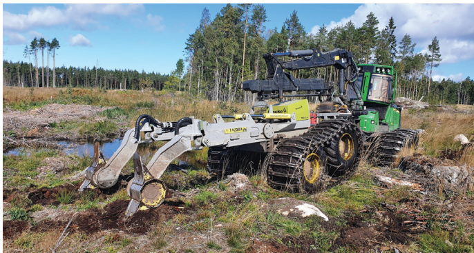
On a medium-sized forwarder, the Bracke M24.a provides very good scarification results on all mounding sites.
