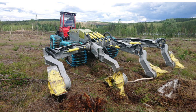
Scarification with the M46.b gives plants and seeds the best possible start for growth and survival whatever the terrain.
