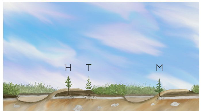
The Bracke M46.b creates planting spots with inverted humus (T), mineral soil mounds on inverted humus (H), and mineral soil mounds (M).
