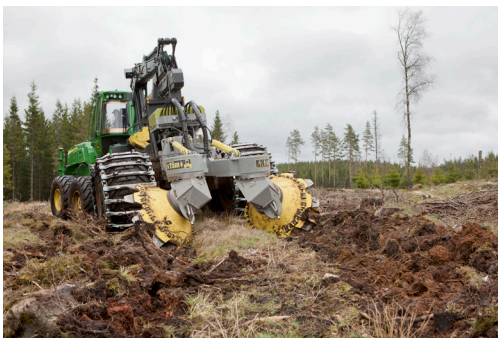
The Bracke T26.b attaches to medium-sized or large prime movers.
